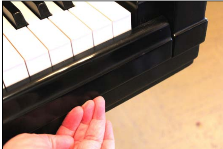
Lifting the Keyslip
